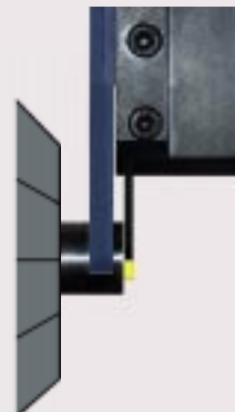
PULLEX advances a little behind the bar centre for gripping the bar
